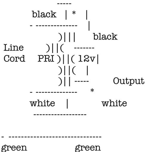
\* Switch the 12 volt leads if output is higher than line!
