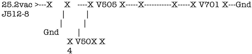
disconnect wire on add new wire pin 7 from pin 3 of V505 and connect to 6.3 v on pin 4 it to gnd. of another tube V50X on IF chassis
