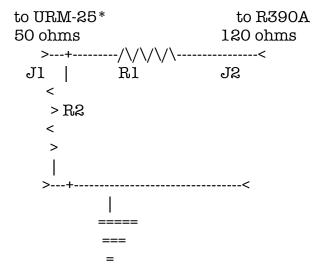
R1 is a 100 ohm 1/4 watt resistor R2 is a 68 ohm 1/4 watt resistor
