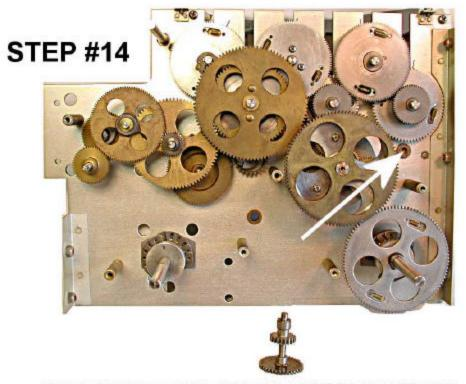
LUBRICATE END OF SHAFT AND SLIDE INTO BRONZE BUSHING.
