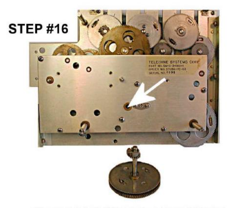
SHAFT WITH CLUTCH ASSEMBLY GOES THROUGH BUSHING AND SMALL GEAR AND CLAMP INSTALL ON SHAFT BEHIND PANEL
