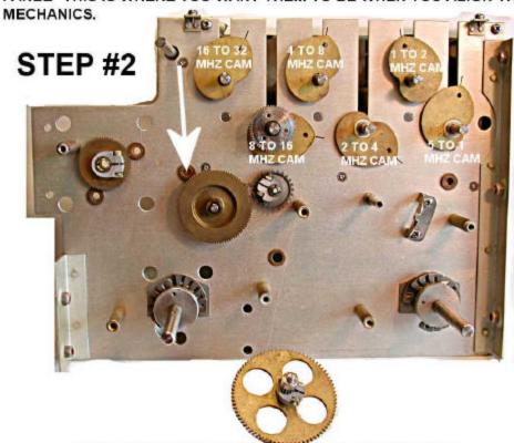
WHITE ARROW INDICATES LOCATION OF THIS GEAR INSERT IT WITH PINION MESHING WITH THE GENEVA DRIVE GEAR
