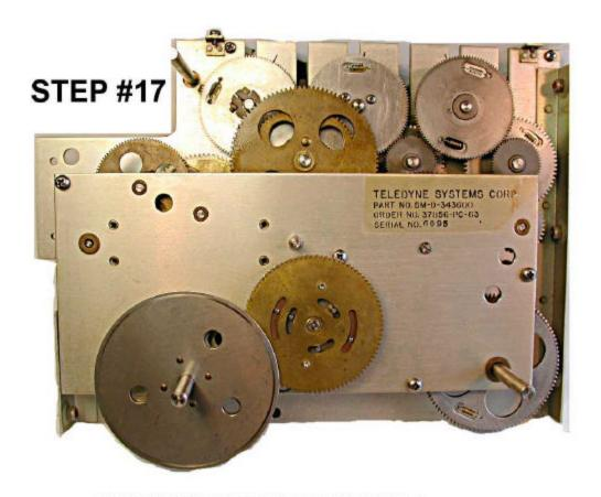
CLUTCH DISK IS CLAMPED ONTO KHZ SHAFT.
