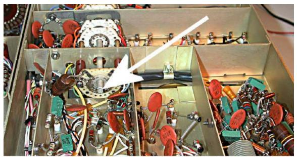
THIS IS THE WAFER OF THE RF BANDSWITCH THAT WE WILL BE LOOKING AT TO MECHANICALY ALIGN THIS SWITCH. IT HAS 6 POSITIONS. THE SWITCH CHANGES POSITIONS WHEN THE MHZ DIAL IS CHANGED FROM: 0 TO 1 MHZ, 1 TO 2 MHZ, 3 TO 4 MHZ, 7 TO 8 MHZ AND 15 TO 16 MHZ. NOTE THAT I SAID THAT THESE ARE THE TRANSITIONS AT WHICH THE SWITCH CHANGES. THE 6 SWITCH SETTINGS REPRESENT THE FOLLOWING BANDS: .5 TO 1 MHZ, 1 TO 2 MHZ, 2 TO 4 MHZ, 4 TO 8 MHZ. 8 TO 16 MHZ AND 16 TO 32 MHZ.
