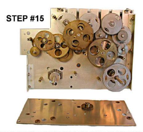
PANEL GOES ON NEXT. CAREFULLY ALIGN SHAFTS INTO BRONZE BUSHINGS ON PANEL TIGHTEN ALL SCREWS GRADUALLY AND EVENLY.
