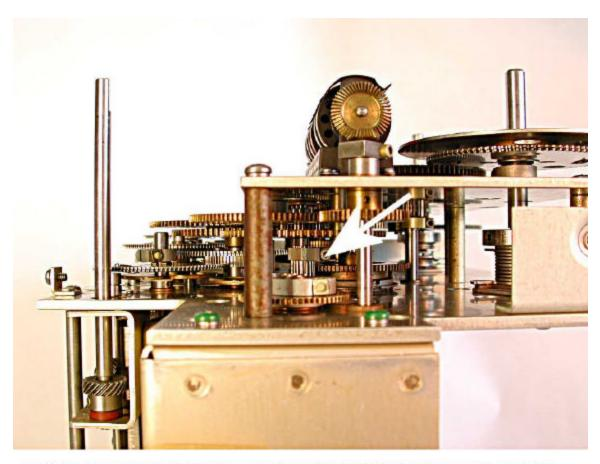
THIS IS THE CLAMP THAT YOU NEED TO LOOSEN IN ORDER TO ADJUST THE RF BANDSWITCH. THE CLAMP HOLDS THE PINION GEAR AS SHOWN IN ASSEMBLY PICTURE #2. YOU NEED TO HOLD THE LARGE GEAR ATTACHED TO THIS SMALL PINION GEAR AND ONLY TURN THE GENEVA DRIVE TO SET THE RF BANDSWITCH.
