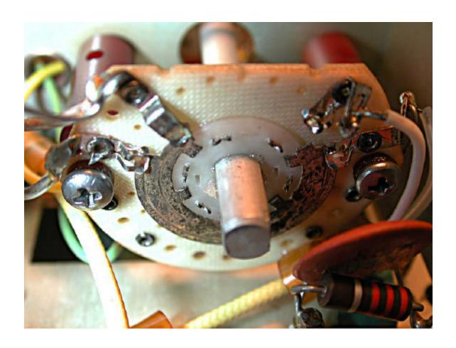
THIS IS THE POSITION OF THE RF BANDSWITCH REARMOST CONTACTS WHEN THE DIAL IS SET IN THE 07 MHZ POSTION. THE KHZ DIAL HAS NO EFFECT ON THIS SWITCH SETTING.
