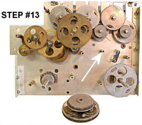
SLIDE GEAR ASSEMBLY ONTO SHAFT SMALL GEAR FACING INWARD.
