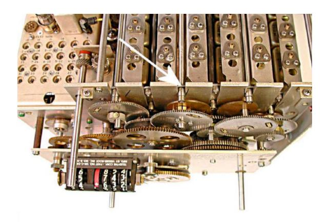
LUBRICATE SLIDES WITH MOBIL 90 WEIGHT SYNTHETIC OIL LUBRICATE ALL GEARS WITH MOBIL 1 SYNTHETIC 30 WEIGHT OIL IT IS IMPORTANT TO USE SYNTHETIC OIL BECAUSE IT WILL NOT DRY OUT AND HARDEN WITH AGE. THE GEARTRAIN WILL NEED TO BE LUBRICATED EVERY 6 MONTHS TO 1 YEAR NEVER USE GREASE. IT WILL JUST MAKE A BIG MESS.
