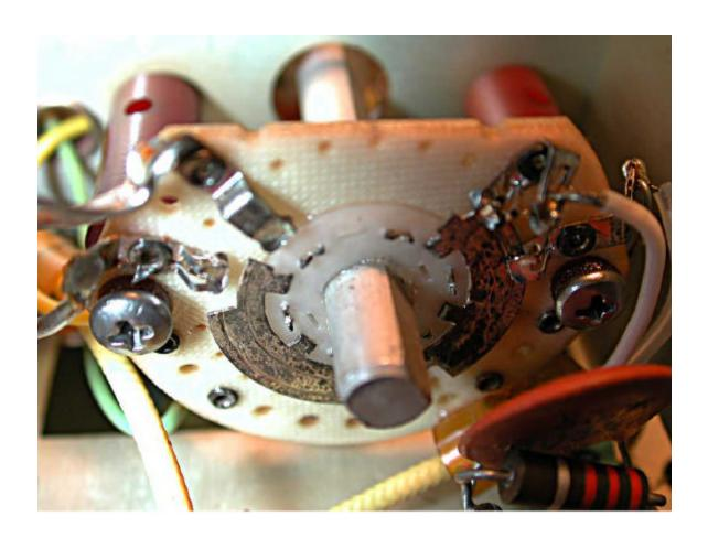
THIS IS THE POSITION OF THE RF BANDSWITCH REARMOST CONTACTS WHEN THE DIAL IS SET IN THE 08 MHZ POSTION. THE UPPER LEFT CONTACTS SHOULD OPEN UP AS THE SWITCH IS TURNED FROM 7 MHZ TO 8 MHZ. THERE IS ONLY ONE POSITION OF THE GENEVA DRIVE THAT WILL PRODUCE THIS RESULT.
