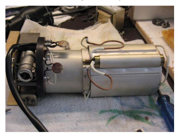
Once the heater unit is removed, you have access to the inner cover. Removing it for the first time after sitting for a long time can be quite difficult, even if the rubber seal is in good condition. As can be seen in the next photo, the seal is about a 1/4" from the base. You might try putting some silicone oil on the joint all around it and let it soak in. Sit it on the end with the electronics end up.
