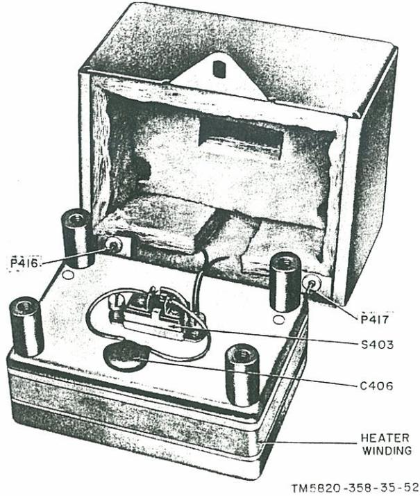
Figure 14. Crystal-oscillator subchassis, internal view of crystal oven.
