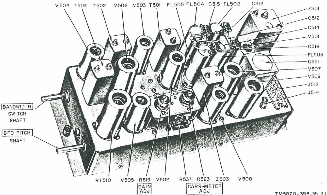
Figure 4. Unmodified IF. subchassis, top view.
