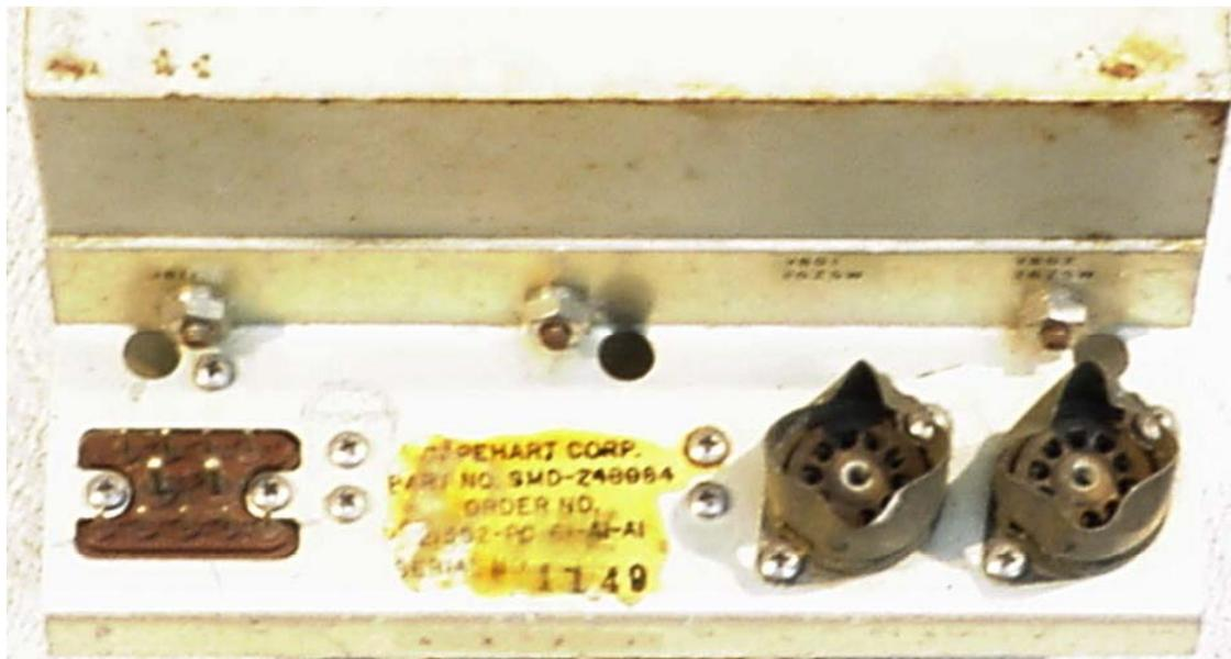
Shown with V801 and V802 replaced with CR801 and CR802 (under sockets) by Field Change 6.
